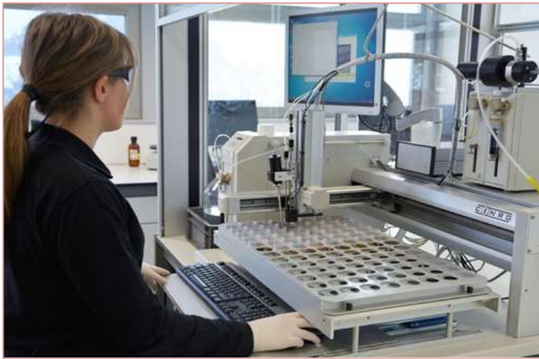
Figure 1: The CINRG CS-APC-2 fully automated auto-diluting particle counting instrument with Klotz LDS Sensor, Klotz USB counter, Baumer UNKC sample level sensor, Gilson 215 liquid handler and CINRG Systems controller.
