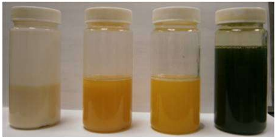
Figure 5: Routine oil samples from the WearCheck laboratory containing high concentrations of free and emulsified water as received and after shaking.
