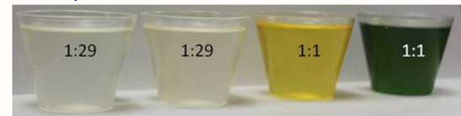
Figure 5 – 0.1% water contamination using 100% toluene as a diluent vs. 0.5% water contamination using 75% toluene / 25% isopropanol as a diluent.
